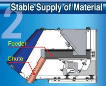
Feeder supply system enables fine adjustment of feeding amount.
