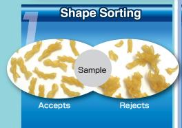
Shape Sorting enables the machine to sort the material by shape (such as broken or adhered) which conventional color sorters could not achieve.
